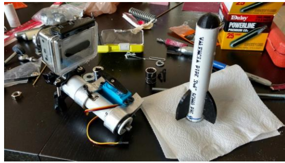
Fig. 5. PVC torpedo and 3D printed head and fins
